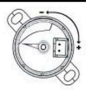
It is possible to carry out a small change of the kilometre number that can be driven as reserve; by rotating the sensor in the seat of the multivalve in counterclockwise direction, the kilometres that you must drive as reserve are reduced, while rotating it in clockwise direction, they increase.
