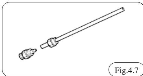
**4.4.5.4 MAP hose (diameters: I.D. 5mm; O.D. 10.5mm)**
